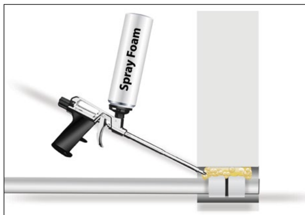
Figure 9.35 Incorrect Placement of Spray Foam Insulation Directly on Polymer Fitting
