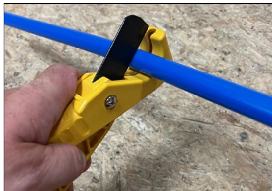
Figure 9.23 Typical PEX Tubing Cutter
