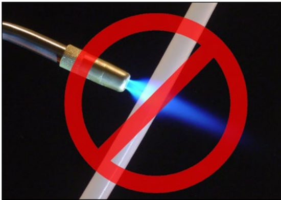
Figure 9.56 Inappropriate Use of Flame on PEX Tubing
