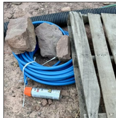
Figure 9.3 Objects that Can Damage PEX
